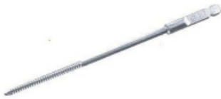
Tap for 2.7mm Cortex Screws Predrilling: 2.0mm dia.
